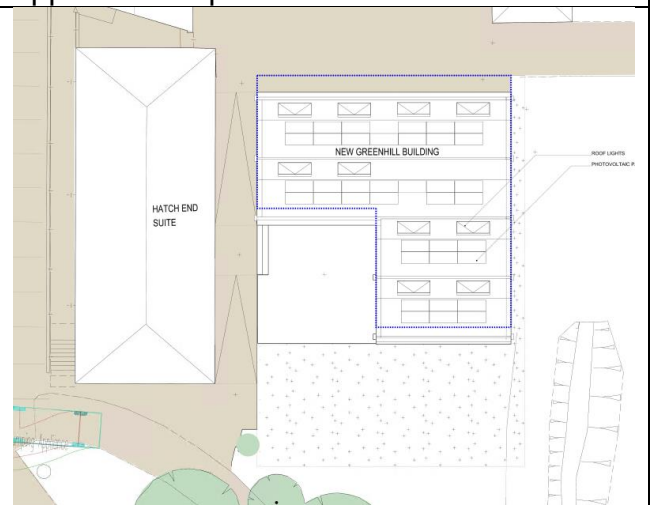
As-built roof plan (blue outline shows approved footprint)
